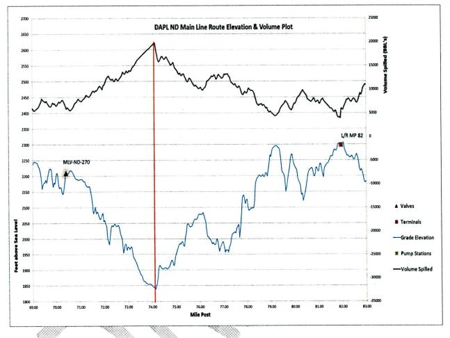
The largest calculated volume occurs at milepost 74.13 miles. Based on the ultimate pipeline flowrate of 600,000 BPD, the volume would be 19,809 barrels of oil. The volume would be reduced to 18,872 barrels based on the initial flow of 450,000 BPD through the pipeline.
